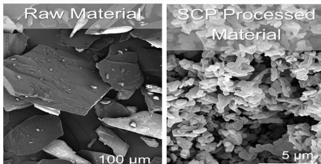
Figure 1. Example SEM Photomicrographs before and after SCP processing.
